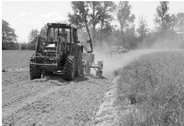
Figure 2 Emission of contaminated dusts during sowing of maize on adjacent crops (picture by the Landwirtschaftliches Technologiezentrum Augustenberg (LTZ))
